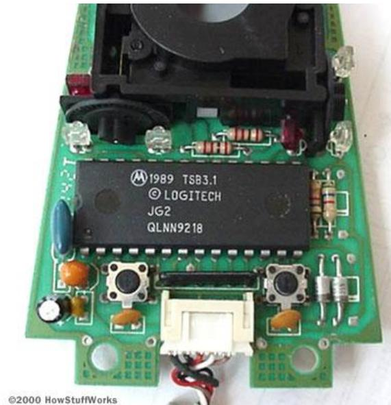
**Fig 2.6 The logic section of a mouse is dominated by an encoder chip, a small processor that reads the pulses coming from the infrared sensors and turns them into bytes sent to the computer. You can also see the two buttons that detect clicks (on either side of the wire connector).**
