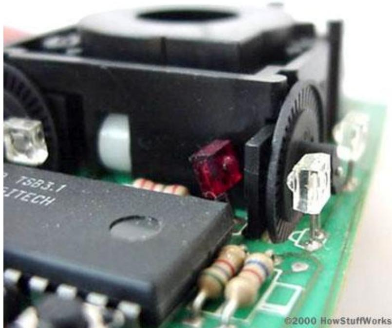
**Fig.2.5 A close-up of one of the optical encoders that track mouse motion: There is an infrared LED (clear) on one side of the disk and an infrared sensor (red) on the other.**
