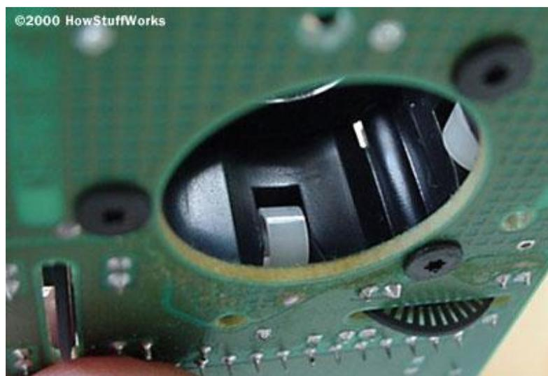
**Fig.2.3 The rollers that touch the ball and detect X and Y motion**
