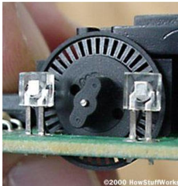
**Fig.2.4 A typical optical encoding disk: This disk has 36 holes around its outer edge.**
