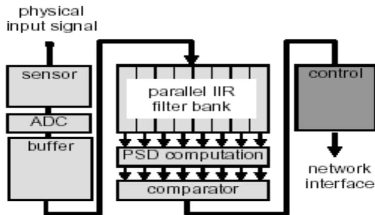
Fig.13 WINS micro power spectrum analyzer architecture.
