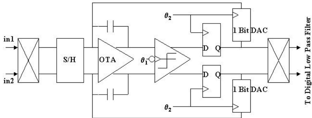
**Fig.8. WINS S-D ADC A block diagram of the pulse code modulator**
