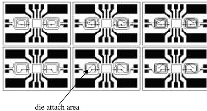
**Fig.15 Low temperature co-fired ceramic layout of (40 nH) inductive loads for the micropower embedded radio**
