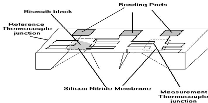
**Fig.6 Thermal Infrared Detector**
