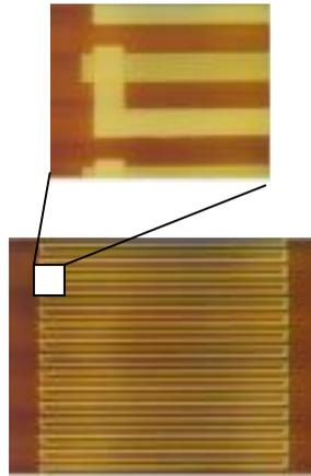
**Fig.7 A Micrograph of the Thermopile Junction Array**
