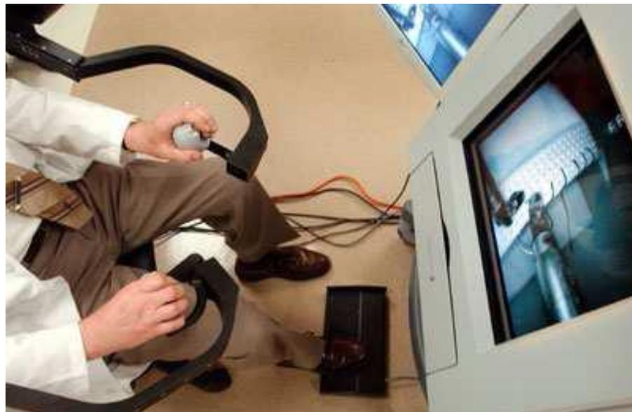
*Fig 3.1 Demonstration of a supervisory-controlled robotic system.*
